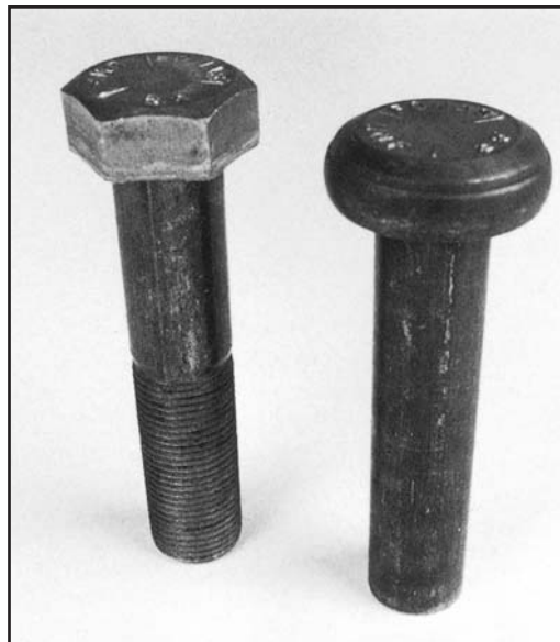
Screwbolt forged in an ASP 23 tool.
