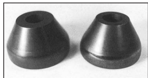
PVD coated tools in ASP 23 for cold forming of tubes.
