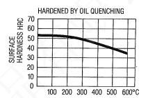
TESTPIECE HARDENED BY OIL QUENCHING FROM 850°C.
